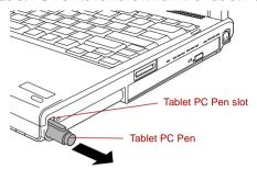
Figure 4-3 Removing the Tablet PC Pen
